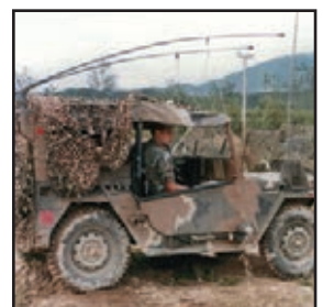
Antenna Tie Down
